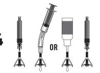
Add sealant: Once successful with inflation remove the valve core to add Stan's sealant. Add 2–4 oz. of sealant. Inflate to riding pressure. Always review the maximum pressure information listed on both the rim and the tire and consider the lower of the two numbers your maximum pressure. Do not inflate above the lower of the two numbers.
