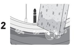
With a brush or sponge apply a generous amount of soapy water to both beads of the tire to help it slip onto the bead of the rim when inflating.
