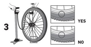
Rotate the valve to 12 o'clock and install a pump. Inflate tire to 35psi to seat tire.
