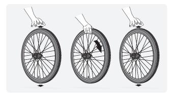
Bounce: hold the wheel vertically and gently bounce or "dribble" it to disperse the sealant throughout the inside of the tire. Let it drop from an inch or two, then rotate a few degrees and repeat. Do this for several revolutions of the wheel.
