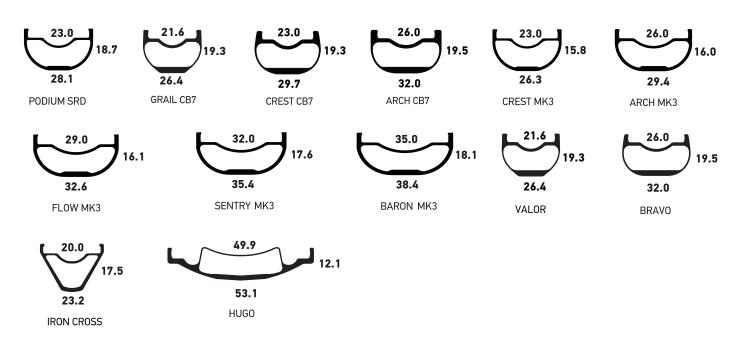
**Caution:** Stan's rims are optimized for tubeless use and designed to set up tubeless with Stan's Yellow Tape, Universal Valves, and Tire Sealant. Tubes may also be used on all Stan's rims; as with all tube installations, care must be taken to prevent tubes from being caught underneath the bead of the tire, causing the tire to dismount when inflated.
