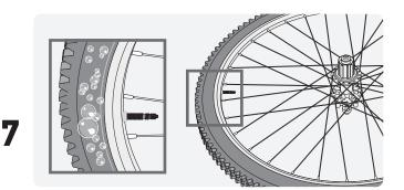
Lay tire on side and apply a thin sheen of soapy water around the sidewall and the bead area. Look for suds occurring anywhere on the tire or bead area. Suds bubbling out from the tire indicate porous areas. Shake the sealant to those areas to seal them and apply soap and water again. Check for suds forming on both sides of the tire. Repeat until no suds remain. Install the cassette and rotors according to the component manufacturer's recommendations.
